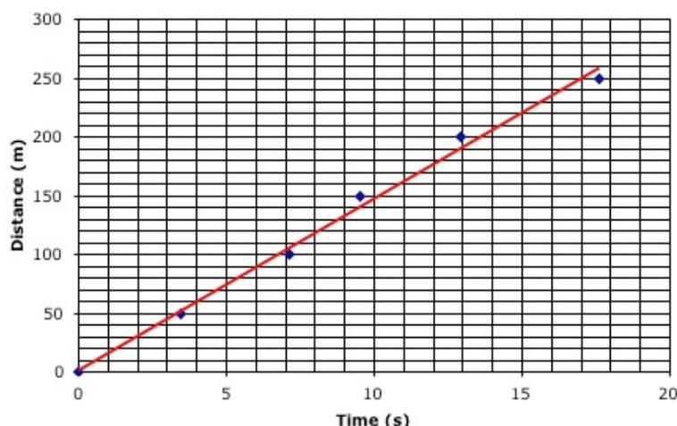
**Figure 1.** A basic correctly scaled and annotated graph. Note the tick marks on both axes, the names of the variables and the units in which the variables are plotted. The points and the trend line are clearly visible. The plot makes good use of the graph area. Note also that this caption is clear and informative.
