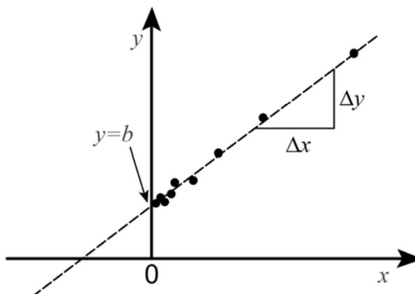
**Figure 3.** A schematic illustration of the linear relationship parameter extraction process. The model equation is linearized, the experimental data is plotted in linearized coordinates, the slope and the intercept are extracted as shown, and then transformed back into physically relevant quantities.
