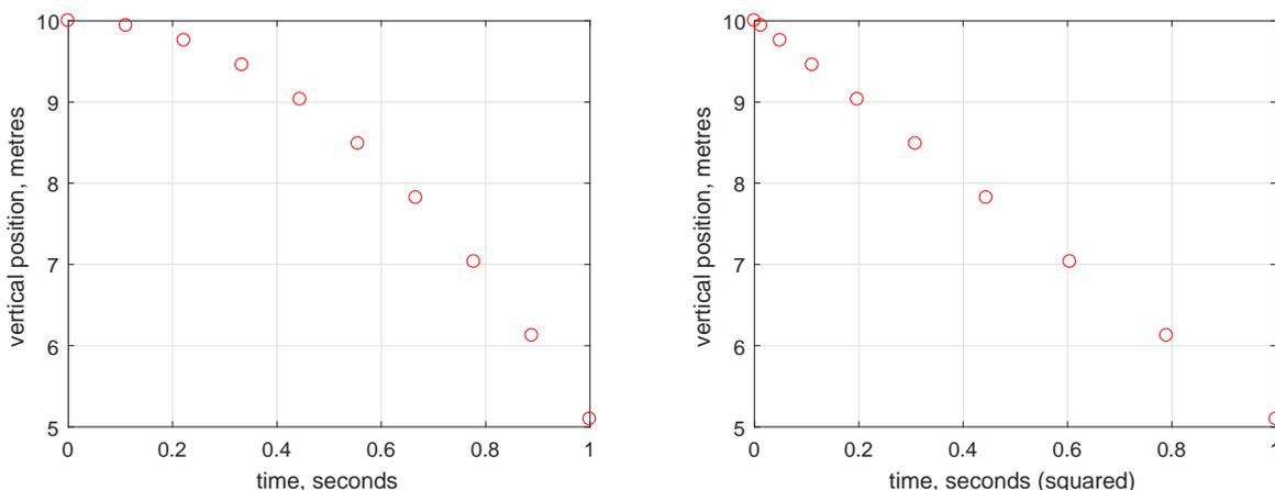
**Figure 2.** An illustration to the fact that the non-linear relationship between the time and the vertical coordinate of a falling object in Equation (2) yields a linear plot when the vertical position is plotted against time squared.
