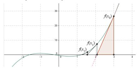
It may be demonstrated that the point  $x_n$  moves closer and closer to the nearest root of f(x) when n is increased. Note that Newton-Raphson algorithm requires an *initial guess*  $x_0$ , that it converges to the *nearest* root to that initial guess and that it may fail to converge if the initial guess is not well chosen.
