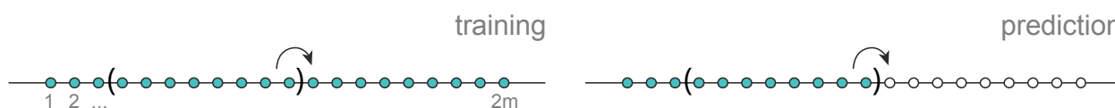
Figure 14. Schematic illustration of training and prediction steps in the linear prediction procedure.
