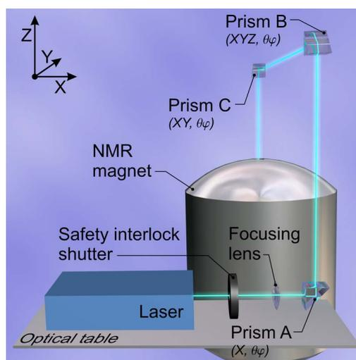
FIG. 2. (Color online) Schematic drawing of the spatial hardware arrangement for the time-resolved photo-CIDNP experiment. Ideally, all three deflectors (prisms or mirrors) should have full rotation and translation stages to facilitate alignment. Minimum requirements for the degrees of freedom are shown in the picture.
